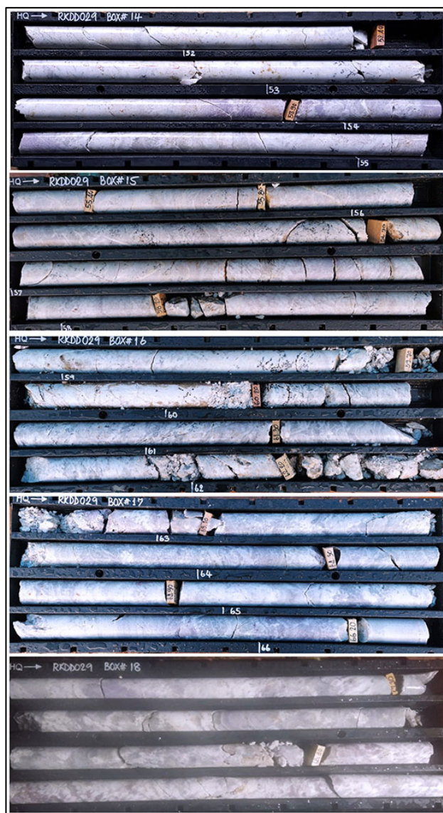
Photo 1. RKDD029 from 51.6m to 70.0m, showing pegmatite with lepidolite
