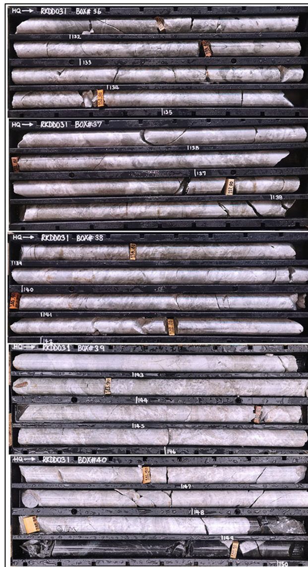
Photo 4. RKDD031 from 138.8m to 149.1m showing pegmatite patchy lepidolite
